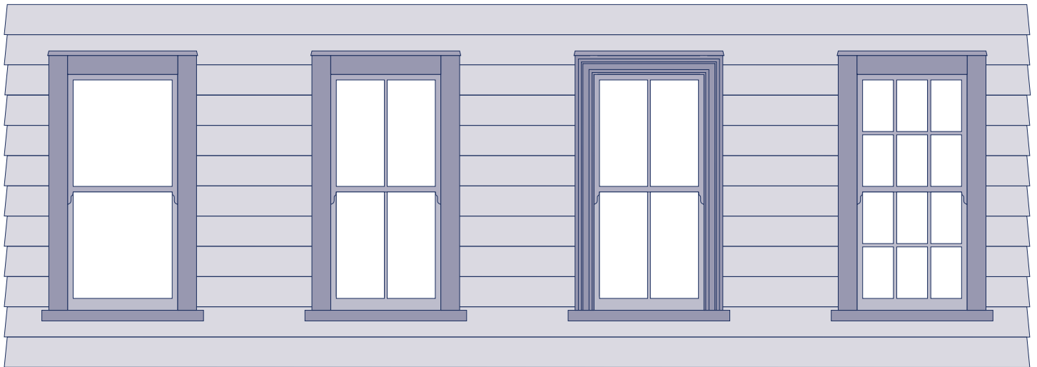
1 Lite Double Hung Window with 140x18mm D4S Facings
